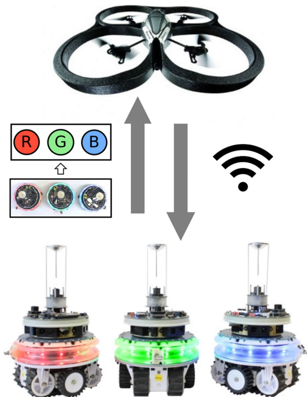
Fig. 2 Our heterogeneous multirobot testbed consists of one AR.Drone (on the top) and multiple marXbots (on the bottom). RGB colors displayed by the marXbots can be detected by the AR.Drone using its downward-pointing camera. Signal transmission to the marXbots occurs over wireless Ethernet
