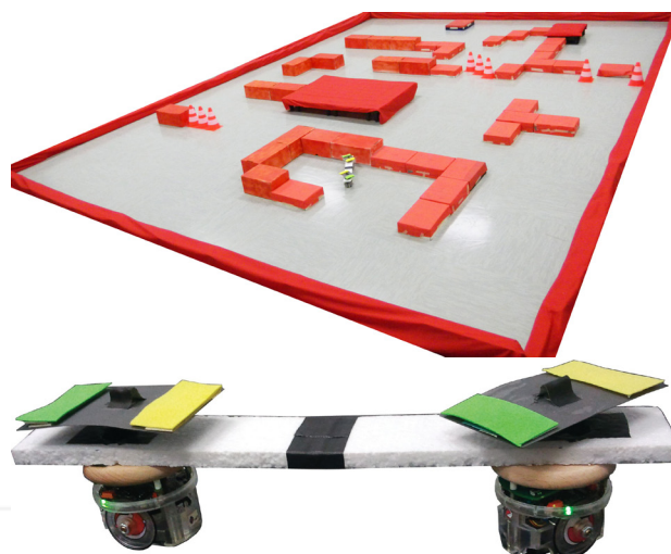
Figure 13. Scenario for real robot experiments. (Top) An example arena. The moving object has to move in the arena while avoiding collisions with the red obstacles. (Bottom) The moving object which follows camera instructions, and which is implemented as a set of two e-puck robots interconnected by a rigid structure.
