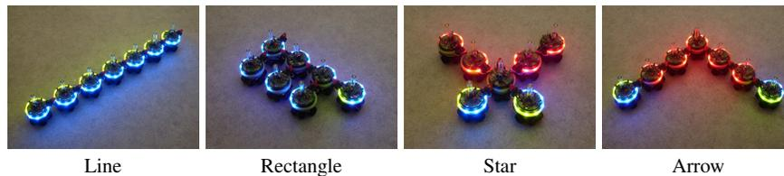
**Fig. 1.13** Four different morphologies constructed with 7 real robots: line, rectangle, star and arrow. Note that the rectangle and star morphologies would become symmetric with the addition of more robots. (Reprinted from [11].)
