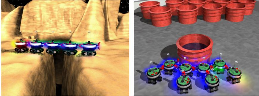
**Fig. 1.1** Two examples of robotic entities self-assembled into morphologies appropriate for the task. Left: A connected robotic entity crosses a gap. A line formation is well-suited to this task, since it allows the entity to stretch further and minimizes the number of robots suspended over the gap. Right: Robots physically connected in a shovel shape to push a heavy object.
