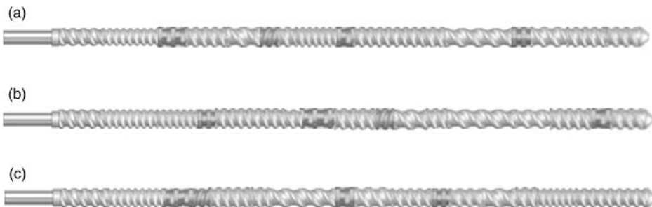
Figure 2. Examples of screw profiles to be used in the extruder of Figure 1.
